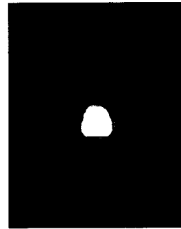
In microgravity, diffusion drives the movement of gases around the flame which becomes spherical in shape.
